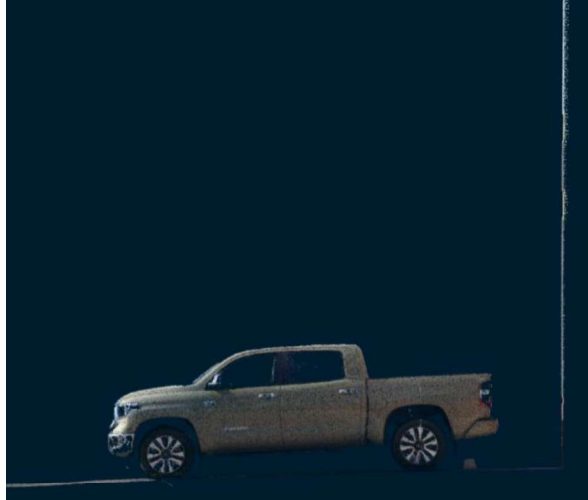
Figure 8: This is a cross section cut of the wall (on right of image) as well as some asphalt from the parking lot as captured by the FARO S150. The vehicle data looks very clean, but there is some reflection noise near the top of the wall due to a combination of the angle of the scan from the ground and the reflective nature of the paint.
