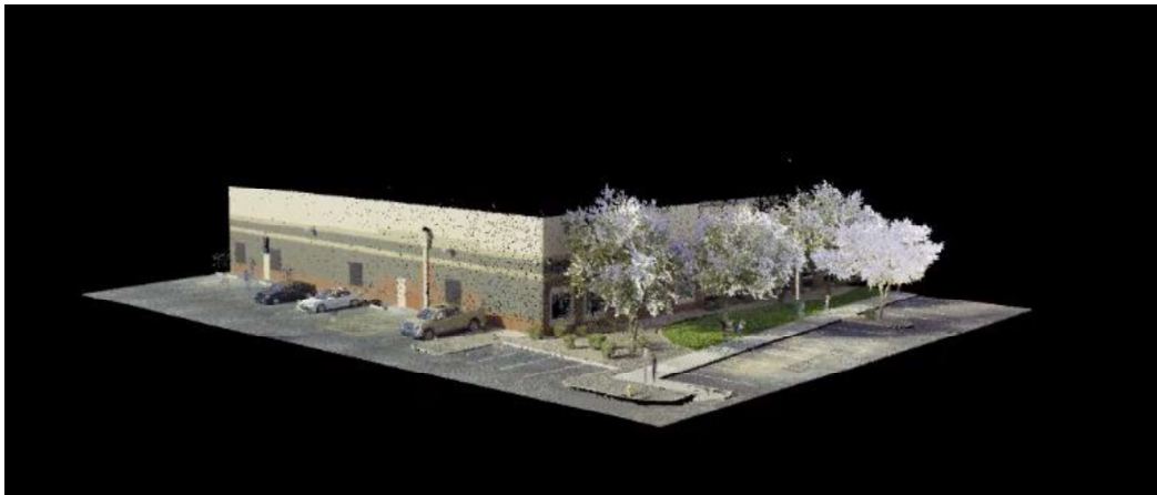
Figure 6: This is a similar comparison for the Leica RTC 360. Please note the darker shades coming from the HDR photos. It is faster with cleaner overall data, but the pixel coloration did not match the field color conditions as accurately as the FARO.
