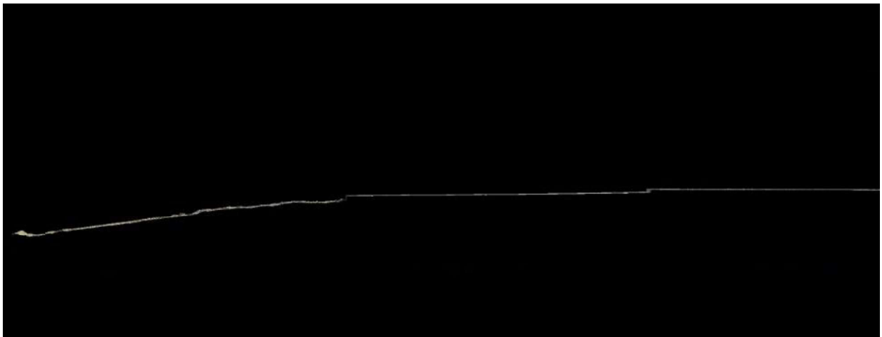
Figure 14: This is a similar cross section from the Leica RTC 360 data. Like the FARO, this non-reflective content produces a sharp edge that is great for floor flatness reports.
