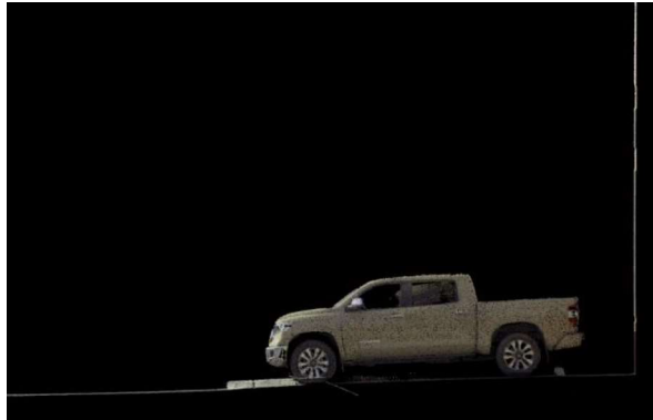
Figure 9: This is a similar slice as captured by the Leica RTC 360. The wall profile is very crisp with no range noise. It is interesting to note that the RTC even captured some content on the rear window of the truck.
