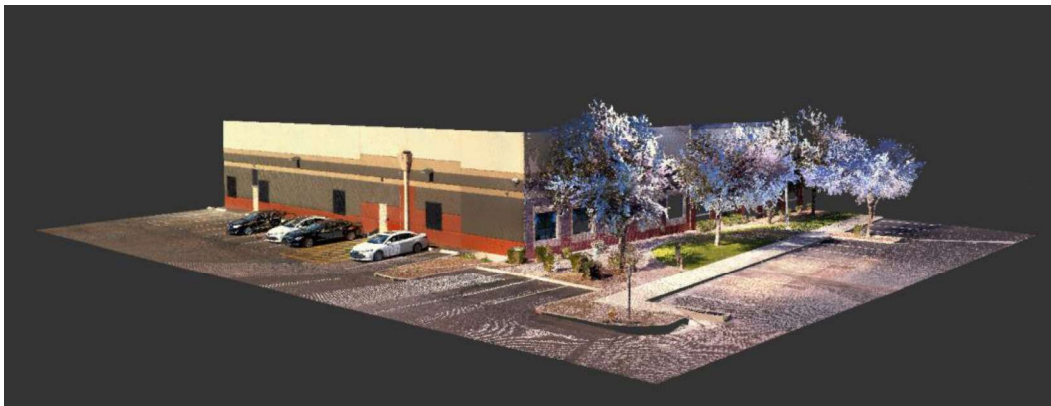
Figure 7: This is the same area as captured from the Trimble X7. Like the Leica, the data is very crisp. The saturation levels are a bit higher than true field conditions, but the higher contrast also makes it easy to identify content particularly on interior scans.
